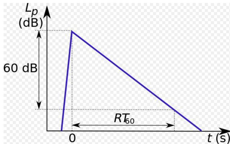
**Figure 1:** Simplified RT60 measurement diagram [10].
