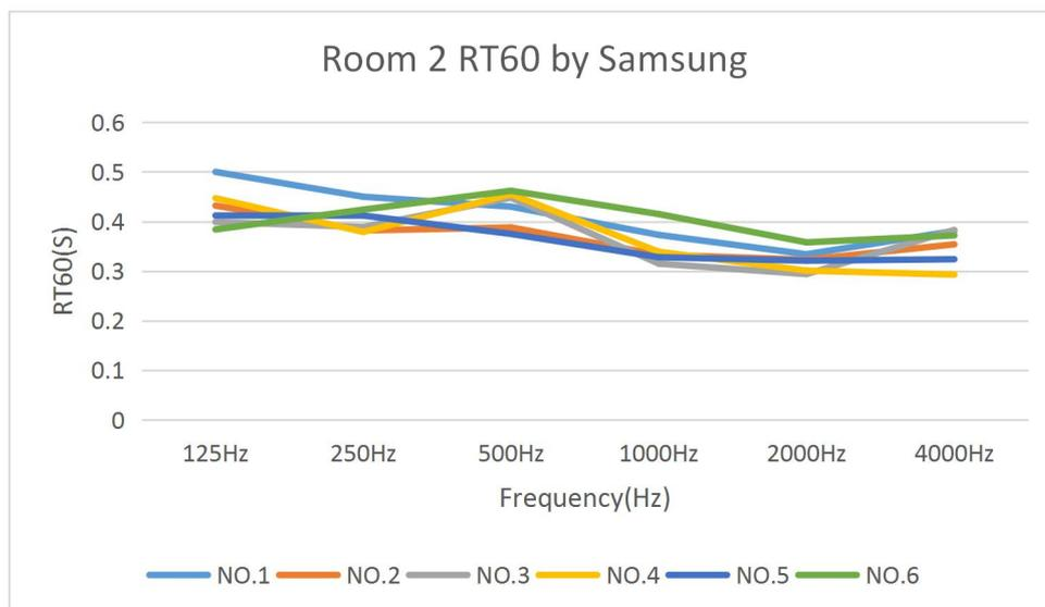
**Figure 30:** RT60 comparison in Room 2 by Samsung.
