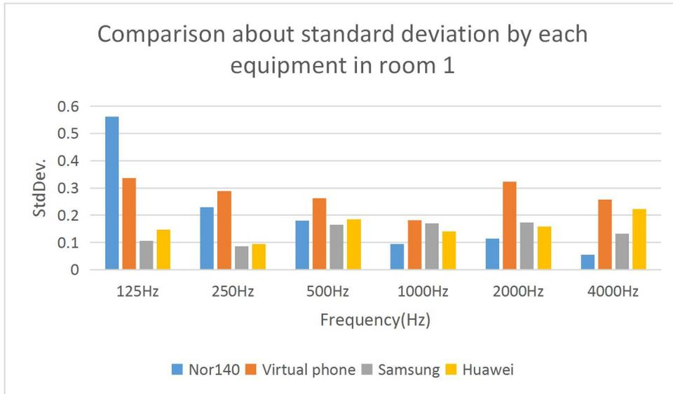
**Figure 35:** Comparison about standard deviation in room 1.
