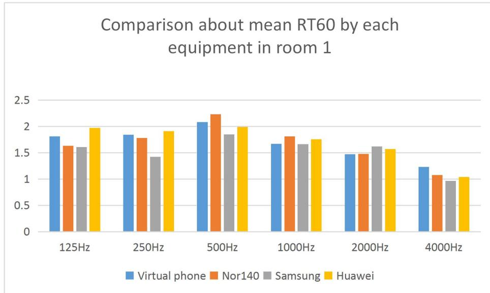
**Figure 33:** Comparison about mean RT60 by each equipment in room 1.
