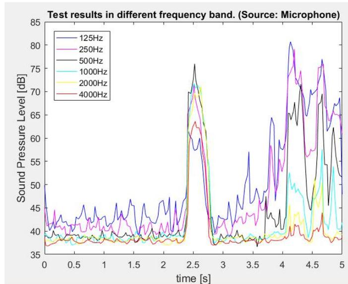
**Figure 14:** SPL-time plot (Microphone as source).
