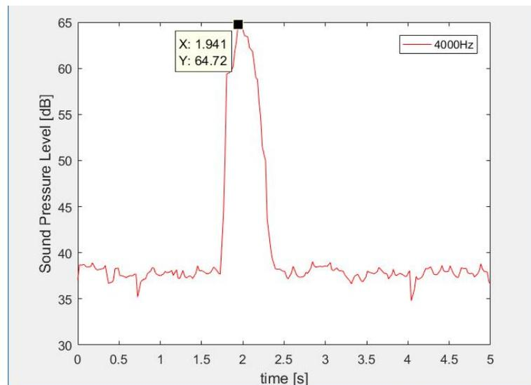
**Figure 18:** Maximum SPL point in 4000 Hz from the example measurement.
