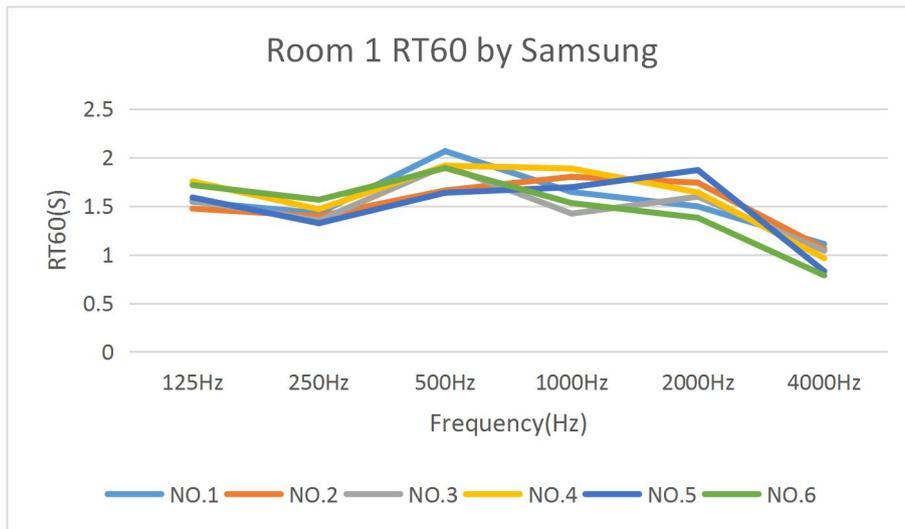
**Figure 29:** RT60 comparison in Room 1 by Samsung.
