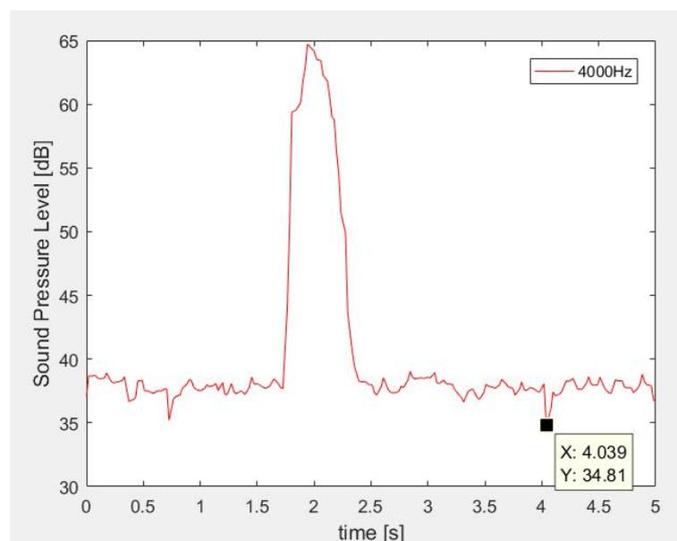
**Figure 20:** The lowest SPL point in 4000 Hz from the example measurement.
