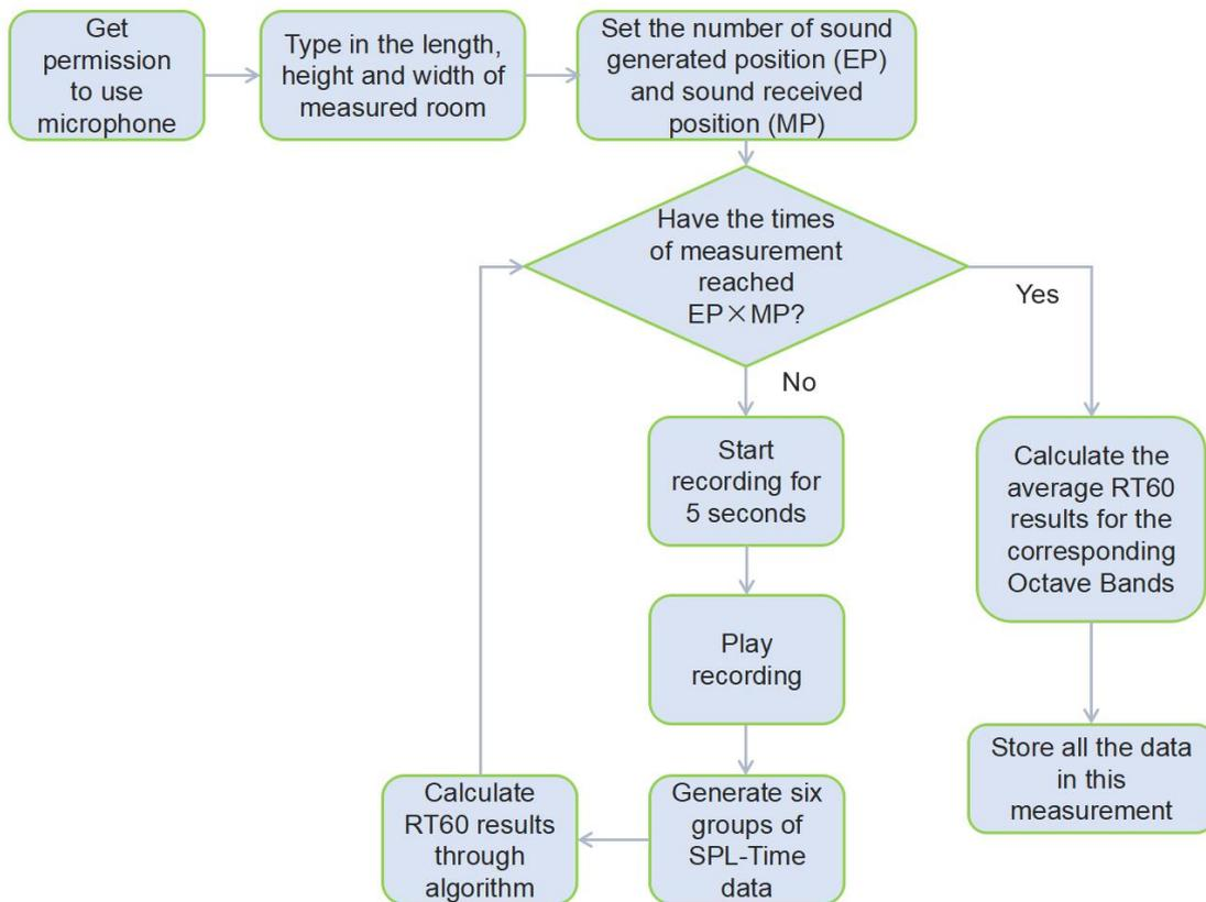
**Figure 9:** Flow chart of the whole measurement process of this app.
