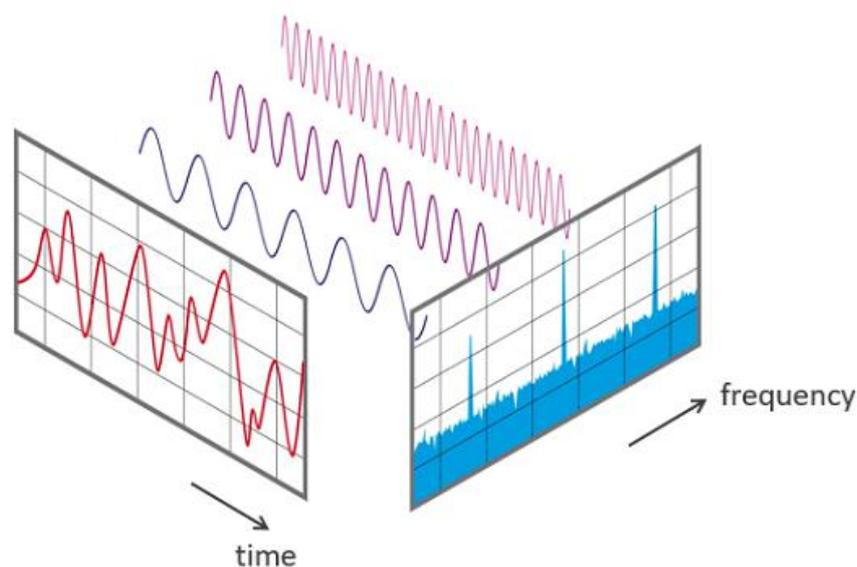
**Figure 3:** Example signal after FFT in time and frequency domain [11].
