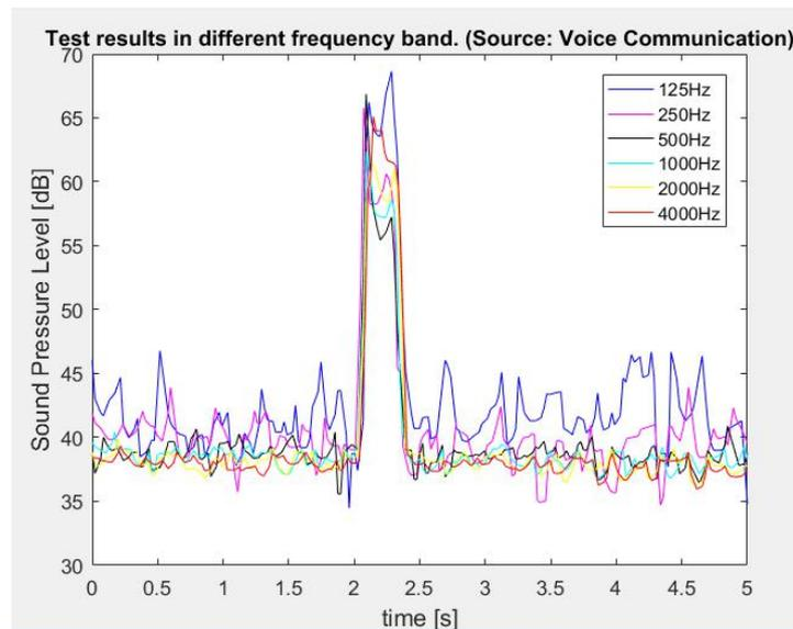
**Figure 15:** SPL-time plot (Voice Communication as source).
