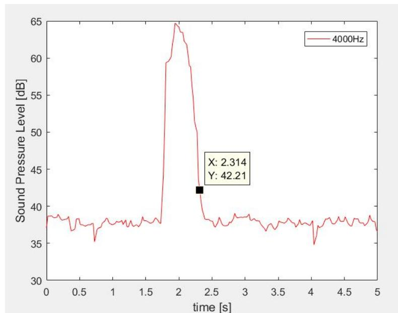
**Figure 21:** The ending point of determined linear decay line in 4000 Hz from the example measurement.
