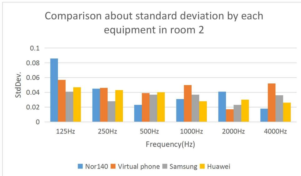
**Figure 36:** Comparison about standard deviation in room 2.
