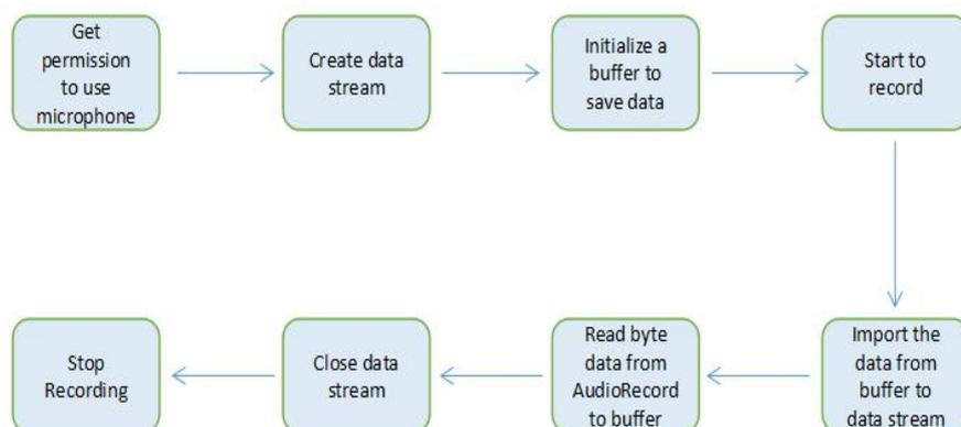
**Figure 10:** Flow chart of sound recording.
