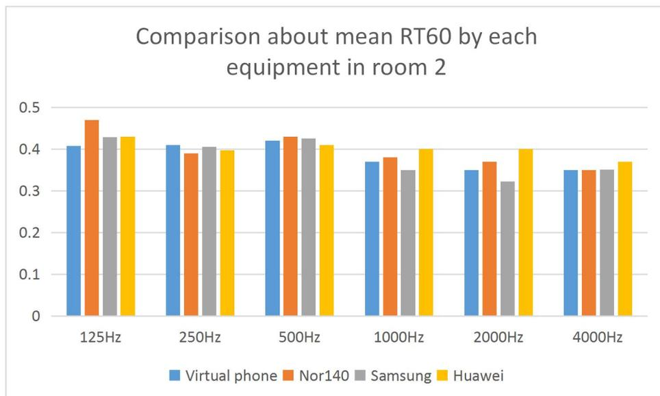
**Figure 34:** Comparison about mean RT60 by each equipment in room 2.
