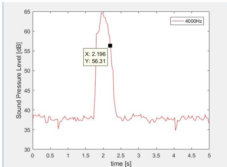
**Figure 19:** The starting point of determined linear decay line in 4000 Hz from the example measurement.
