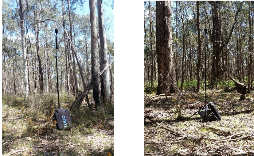
Figure 4.2. Arrangement of DUO meters during forest sound measurements. (a) 300 m. (b) 600 m.
