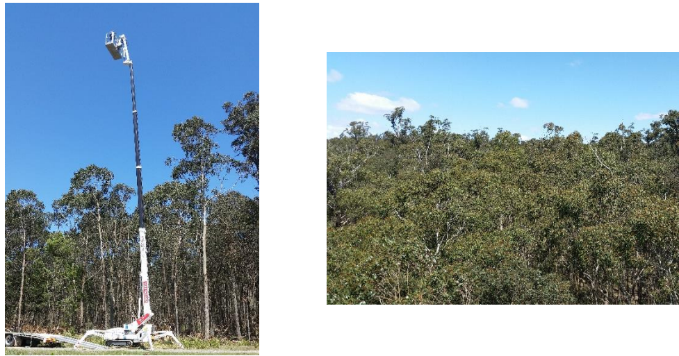
Figure 4.3. (a) The loudspeaker elevated to 26 m above ground. (b) View from the boom lift.
