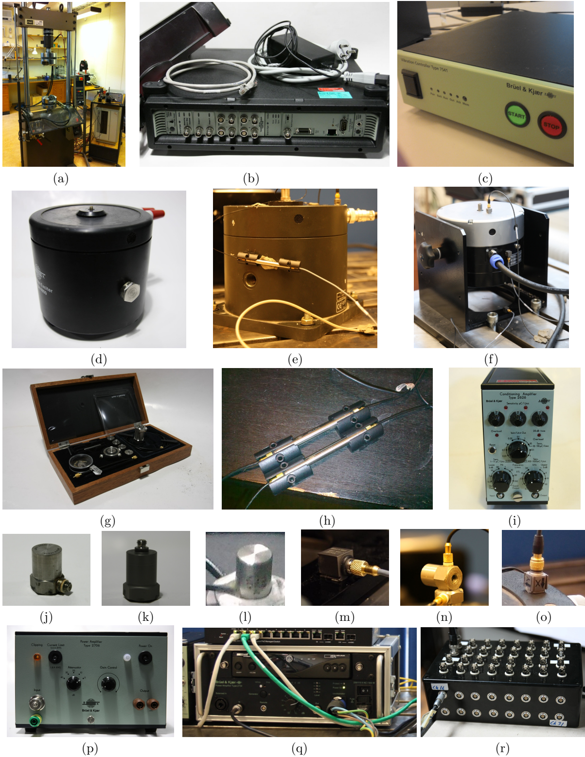
Fig. 4.1: (a) Material testing system MTS 810; (b) Data acquisition system B&K PULSE; (c) Vibration controller B&K 7541; (d) Electrodynamic shaker B&K 4809; (e) Electrodynamic shaker B&K 4808; (f) Electrodynamic shaker B&K 4824; (g) Reference accelerometer B&K 8305; (h) Charge-to-DeltaTron Converter B&K 2647A; (i) Charge amplifier B&K 2626; (j) Accelerometer B&K 4371; (k) Accelerometer B&K 4384V; (l) Accelerometer B&K 4374; (m) Accelerometer B&K 4507 001; (n) Accelerometer B&K 4332; (o) Accelerometer B&K 4524B; (p) Power Amplifier B&K 2706; (q) Power Amplifier B&K 2734; (r) in-house made connection box for MEMS accelerometers (with built-in power supply).
