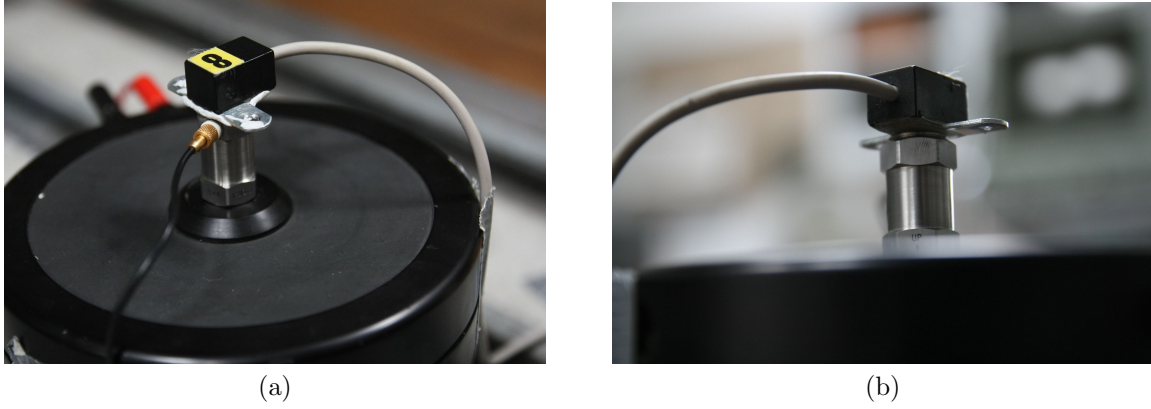
Fig. 7.5: Fixation of accelerometer: (a) using wax; (b) using cyanoacrylate glue.
