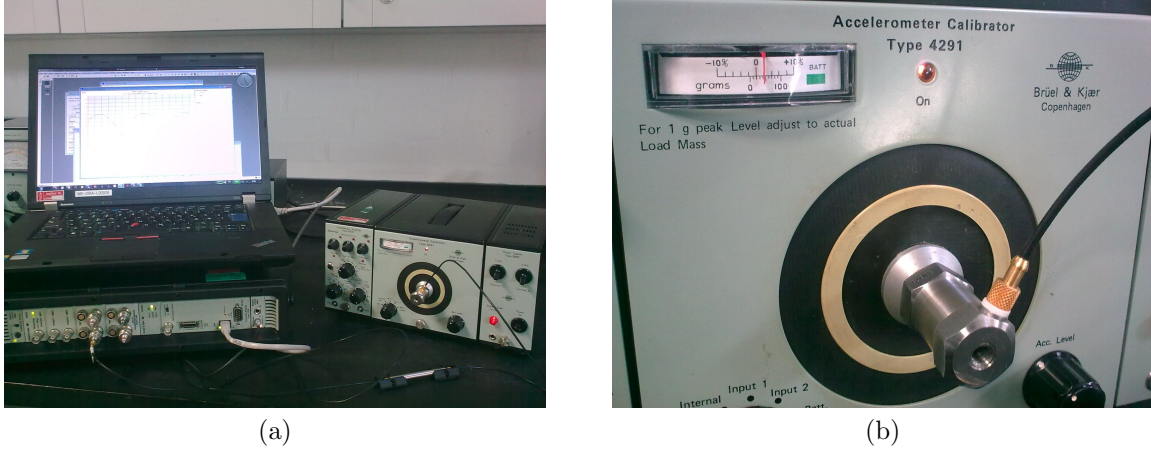
Fig. 6.2: (a) Set-up with B&K 4291 used for the B&K 8305 test calibration; (b) the calibrator B&K 4291.
