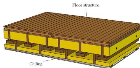
Figure 4: floor element, floor structure and ceiling, made by Martinsons Byggsystem AB.
