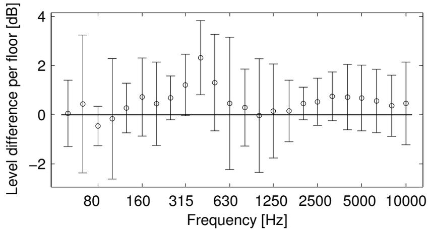
Figure 5: The difference of impact sound insulation between the floors, mean values (circle) and its 95%-confidence limits, for each 1/3 octave band. Positive values means higher impact sound level at higher floor.
