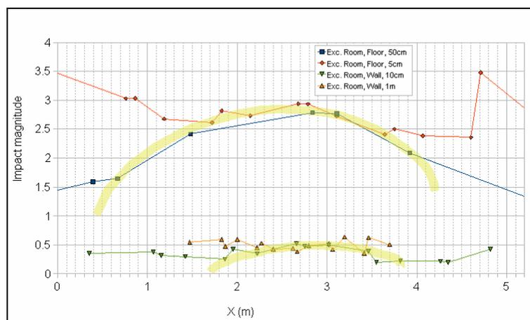
Figure 11: Magnitude of the impact acceleration in the floor, along the wall, as a function of the X-coordinates and corresponding acceleration recorded on the wall in the same room.
