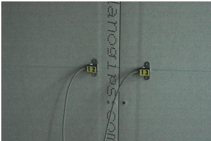
**Figure 7: Accelerometers near a beam on the wall**
