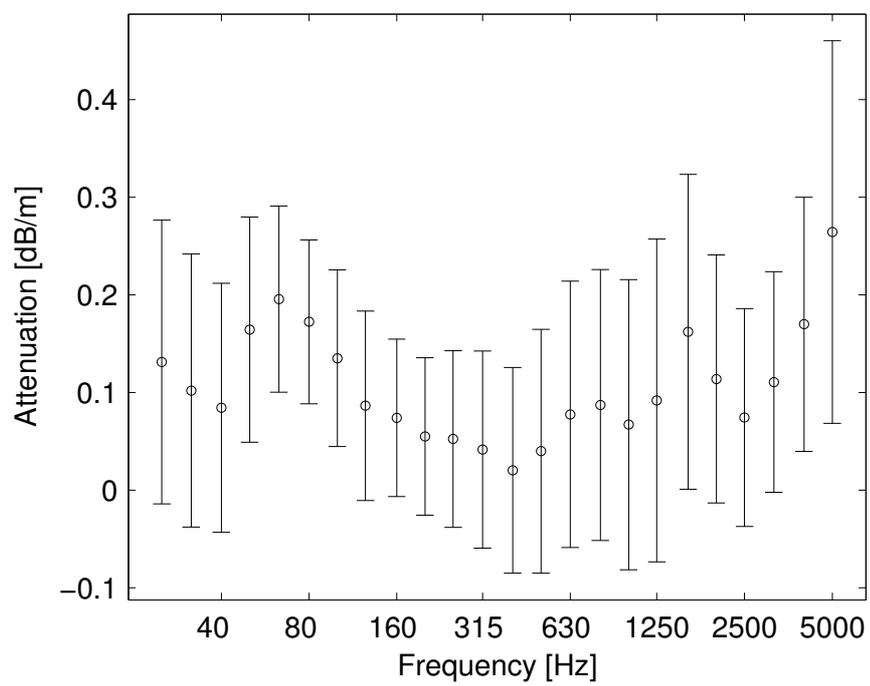
Figure 7: The mean attenuation in the direction along the beams (circle) together with its 95% confidence interval.
