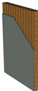
Figure 5: An inner wall containing five layers of massive wood and one gypsum board
