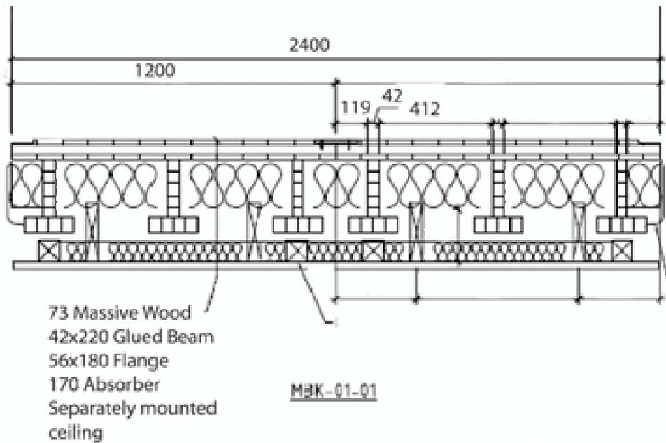
Figure 2: One element of the measured construction. These elements were joined to build the whole floor structure.
