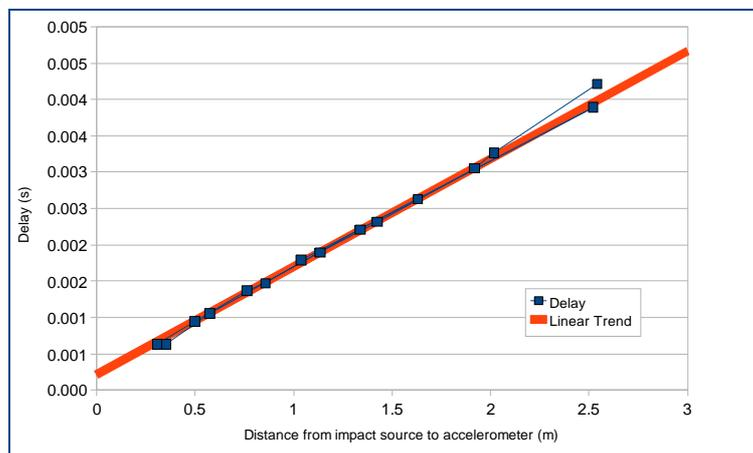
Figure 10: Time delay of the impact acceleration as a function of the distance to the source.
