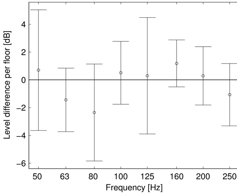
Figure 6: The difference of sound reduction between the floors, mean values (circle) and its 95%-confidence limits, for each 1/3 octave band. Positive values means higher sound reduction level at higher floor.
