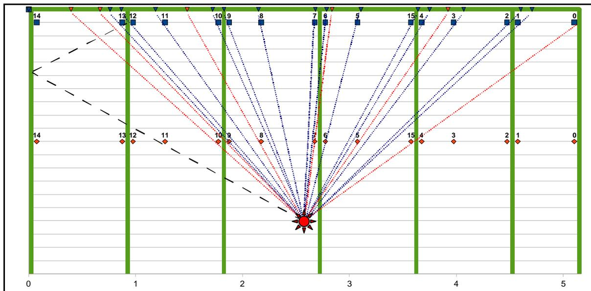
Figure 7: Placement of both lines of accelerometers in the room
