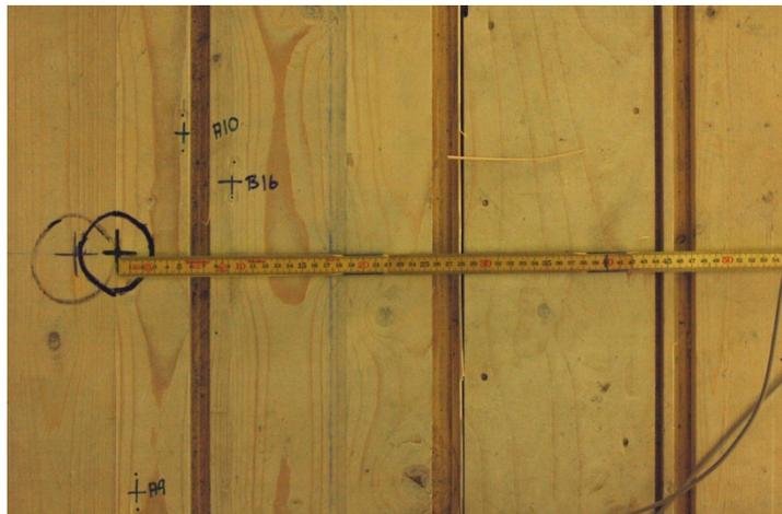
**Figure 2: Distances between hammer impact and accelerometers**
