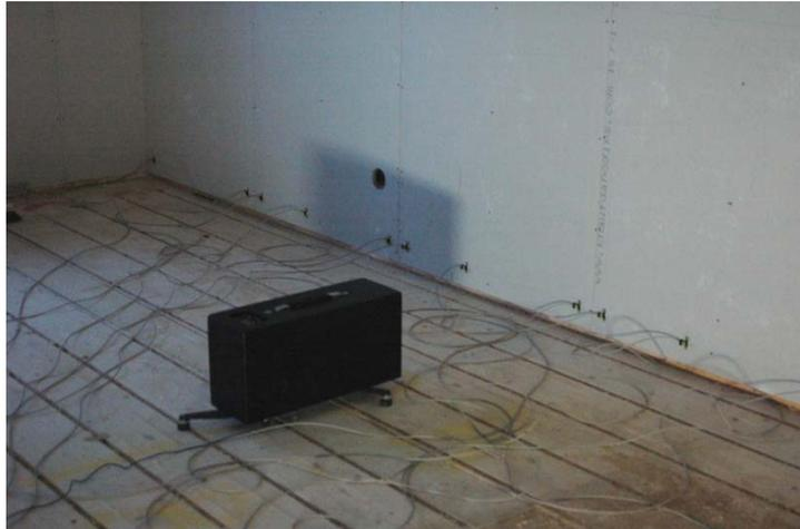
**Figure 4: Hammer in front of the measured wall with 16 accelerometers**
