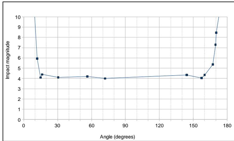
Figure 9: Normalized impact acceleration magnitude as a function of the incidence angle.
