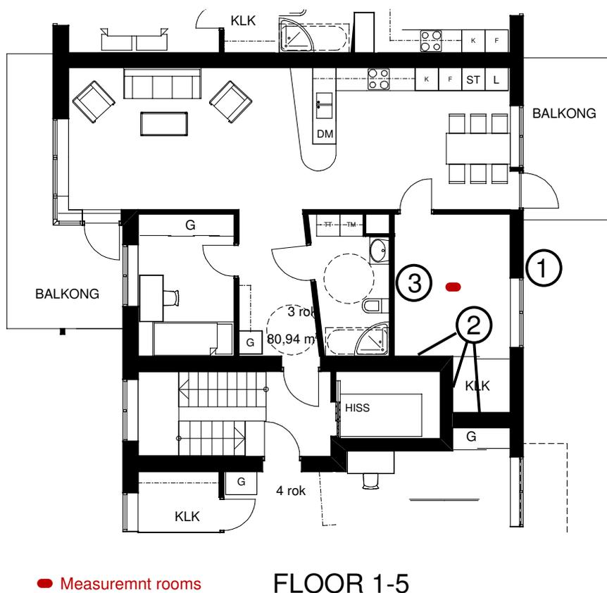
Figure 1: A part of the drawing for the house Linnologen. The sound reduction and the impact noise was measured vertically between the rooms marked in the drawing.
