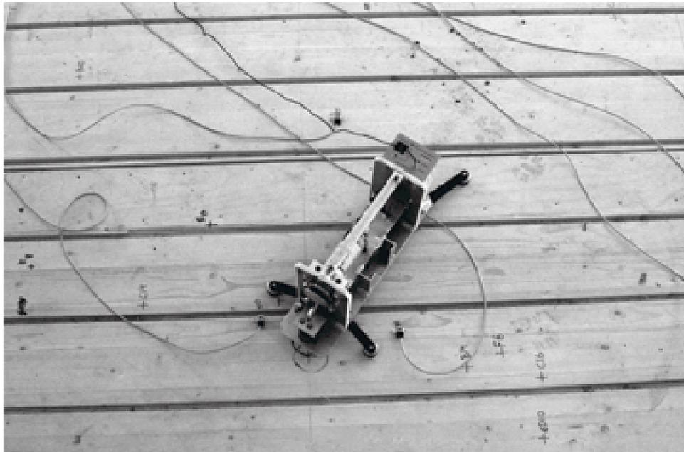
Figure 3: The measurement setup near the point of impact. The picture is taken a bit from above towards the floor structure with the tapping machine. One can also see the traces made in the top plate. Some of the accelerometers closest to the point of excitation can be seen as well.
