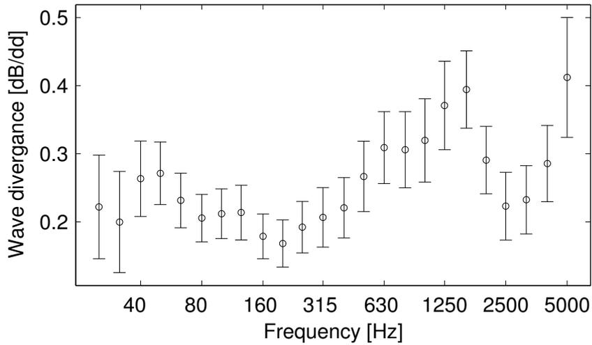
Figure 9: The mean wave divergence away from the excitation and the corresponding 95% confidence interval.
