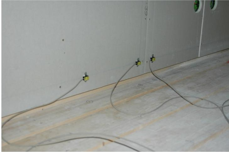
**Figure 6: Accelerometers fixe on the wall**
