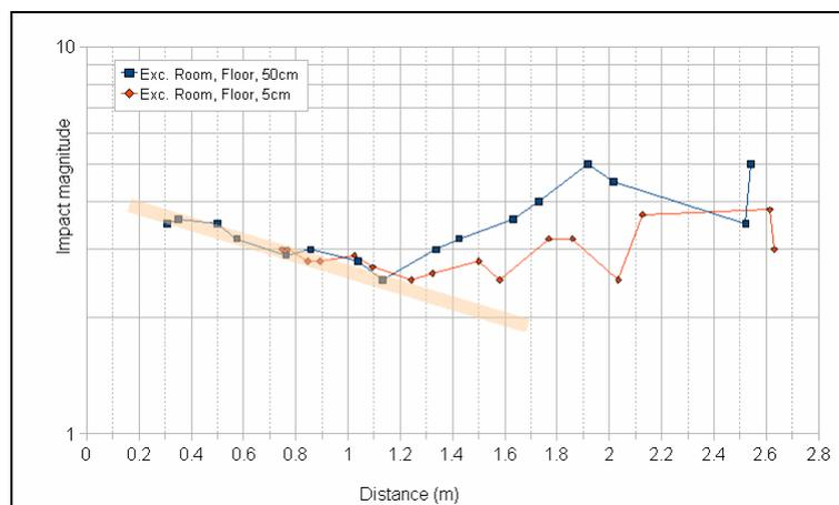
Figure 8: Impact acceleration magnitude as a function of the distance to the source.
