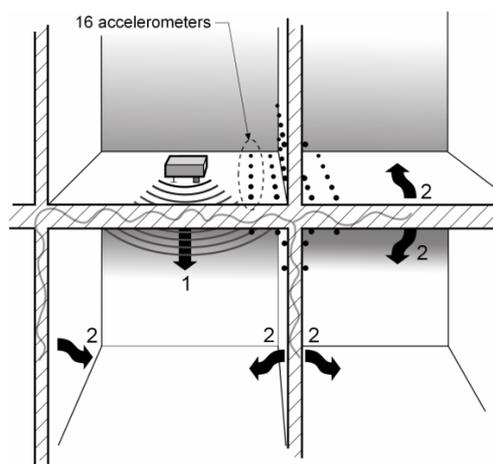
Figure 6: Measurements set up
