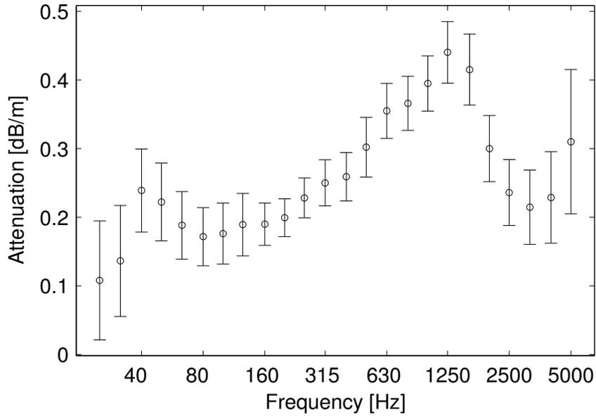
Figure 8: The mean attenuation in the direction across the beams (circle) together with its 95% confidence interval.
