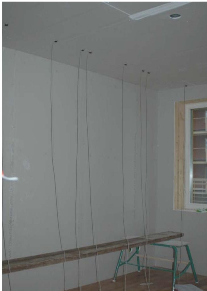
**Figure 5: Accelerometers fixe on the ceiling**
