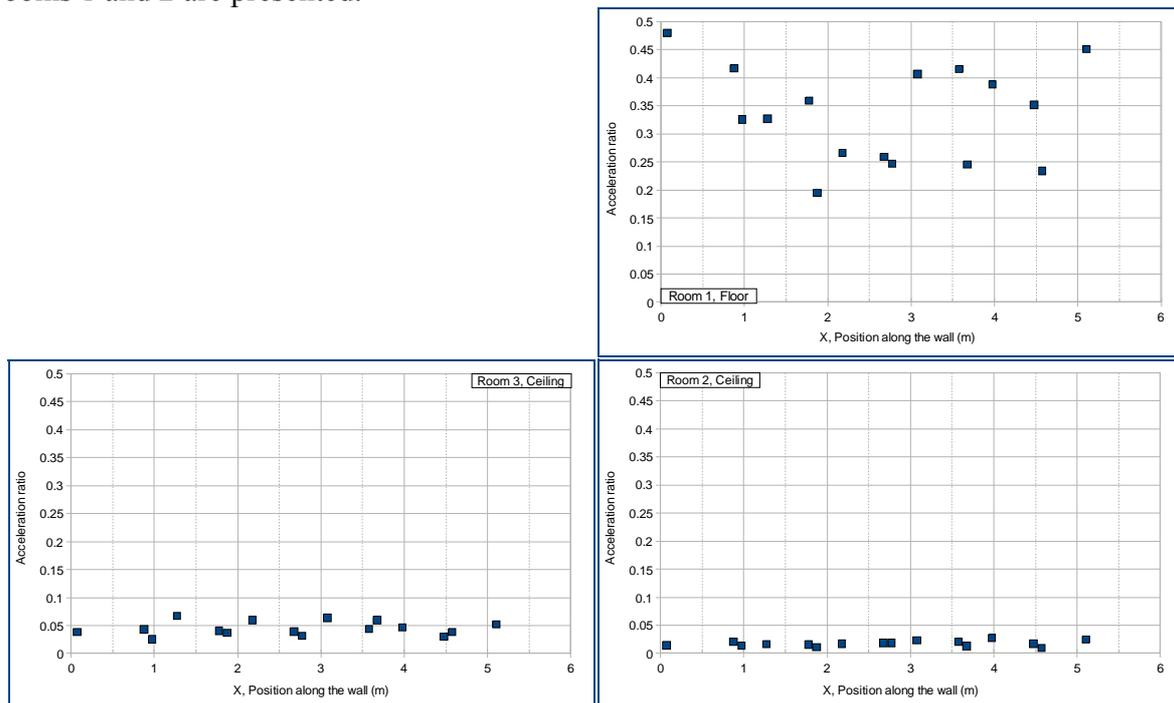
Figure 13: Transmission coefficient of the junction for a impact wave path propagating from the floor in the excitation room to the floor in room 1 (upper right corner) and to the ceiling, in room 2 (lower right) and in room 3 (lower left). The coefficient is defined here as the ratio of the acceleration before and after the junction, and is plotted as a function of the X-coordinates along the junction.
