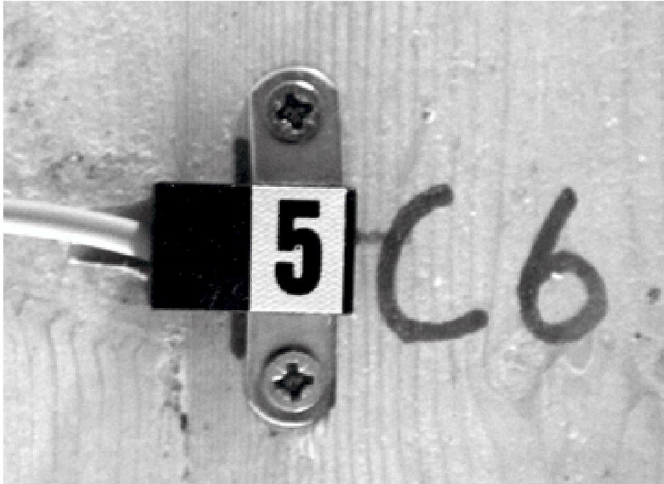
Figure 4: The accelerometers were screwed into place by two screws. The orientation was always the same.
