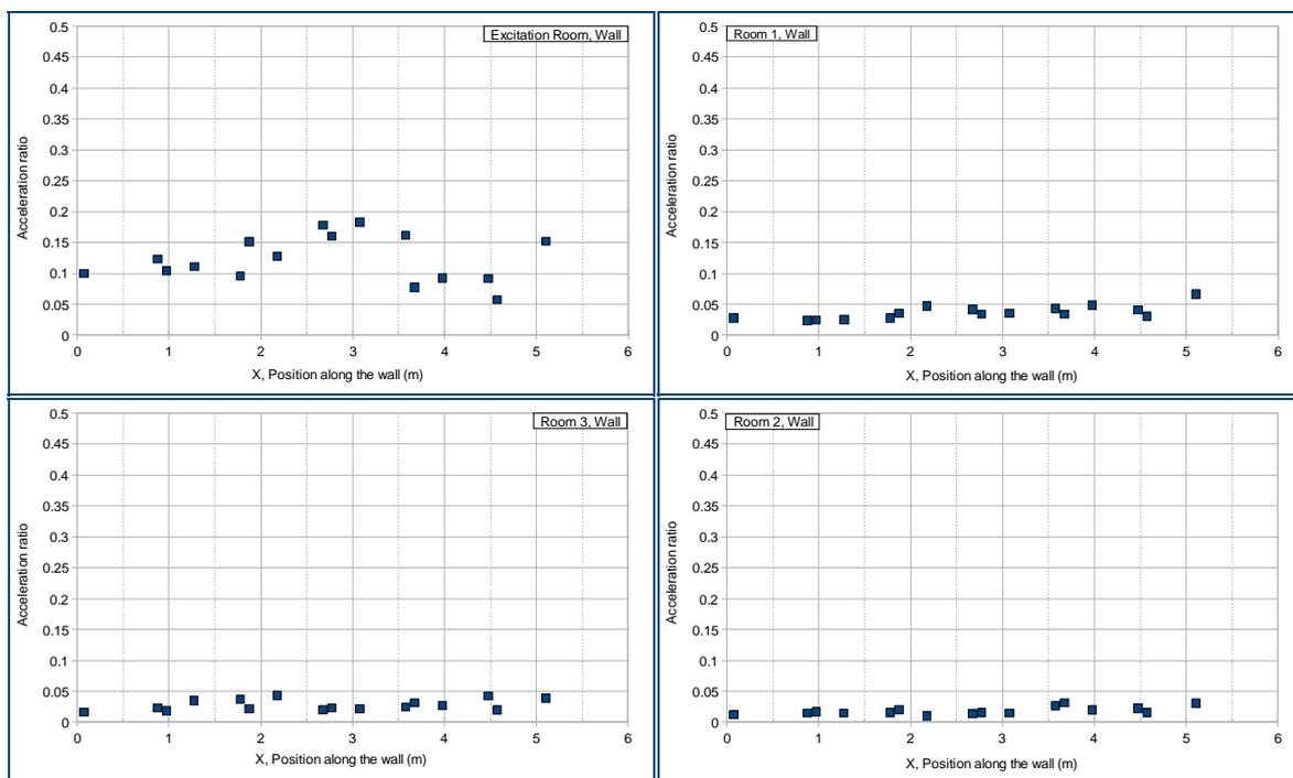
Figure 12: Transmission coefficient of the junction for an impact wave path propagating from the floor in the excitation room to the wall in excitation room (upper left), in room 1 (upper right), in room 2 (lower right) and in room 3 (lower left). The coefficient is defined here as the ratio of the acceleration before and after the junction, and is plotted as a function of the X-coordinates along the junction.
