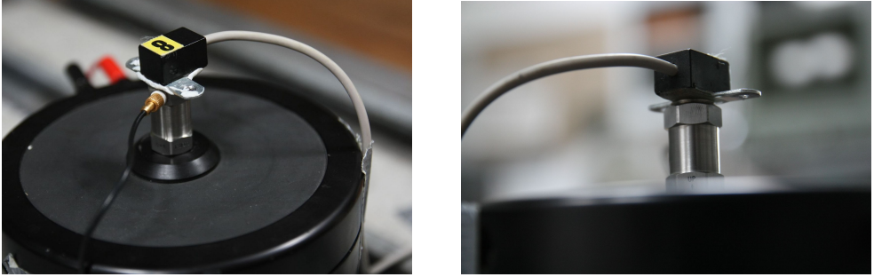
Fig. 7.5: Fixation of accelerometer: (a) using wax; (b) using cyanoacrylate glue.
