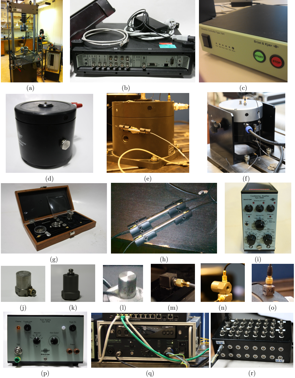
Fig. 4.1: (a) Material testing system MTS 810; (b) Data acquisition system B&K PULSE; (c) Vibration controller B&K 7541; (d) Electrodynamic shaker B&K 4809; (e) Electrodynamic shaker B&K 4808; (f) Electrodynamic shaker B&K 4824; (g) Reference accelerometer B&K 8305; (h) Charge-to-DeltaTron Converter B&K 2647A; (i) Charge amplifier B&K 2626; (j) Accelerometer B&K 4371; (k) Accelerometer B&K 4374; (l) Accelerometer B&K 4507 001; (m) Accelerometer B&K 4332; (n) Accelerometer B&K 4524B; (o) Accelerometer B&K 4524B; (p) Power Amplifier B&K 2706; (q) Power Amplifier B&K 2734; (r) in-house made connection box for MEMS accelerometers (with built-in power supply).
