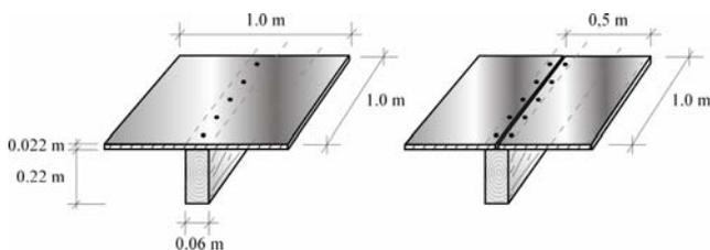
Figure 2: The two models of a beam-plate assembly
