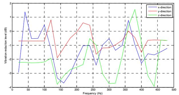
Figure 7: Vibration reduction level in three directions for a rubber layer junction.
