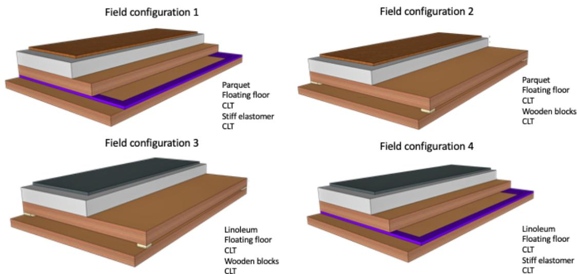
*Selection of configurations tested in factory conditions*
