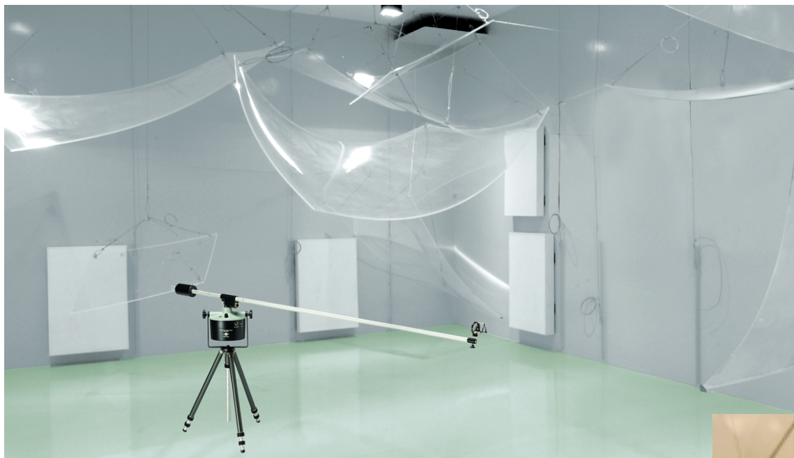
Acoustic laboratory: Reverberation room
