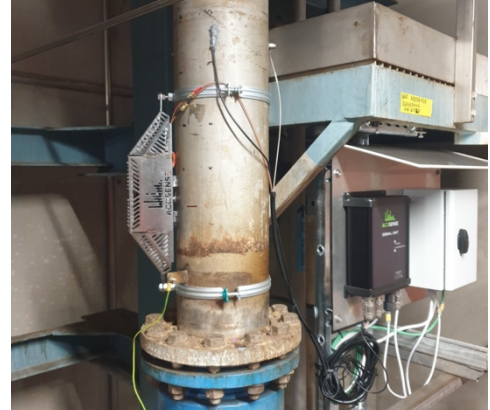
Figure 1: Acosense instrument consists of piezo electric actuators, force transducers and accelerometers installed on the outside of pipes and tanks.
