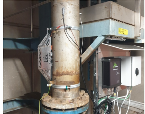
Figure 1: Acosense instrument consists of piezo electric actuators, force transducers and accelerometers installed on the outside of pipes and tanks.
