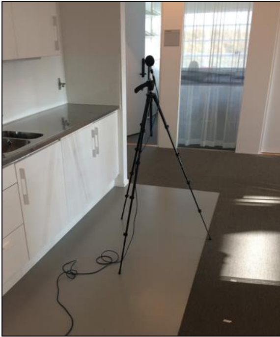
Figure 4.1. Microphone during sound pressure level measurements.
