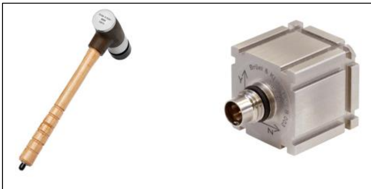
Figure 2.6. An impulse hammer (left) used for exciting vibrations and an accelerometer (right) for collecting the vibration data (Copyright © Brüel & Kjær).
