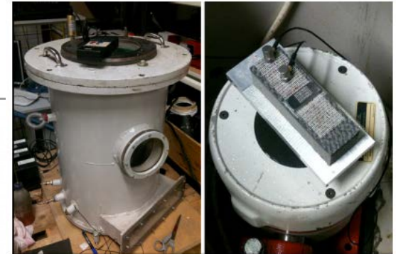
FIG. 3. (Color online) Vacuum chamber and instrumented long sample to the right.
