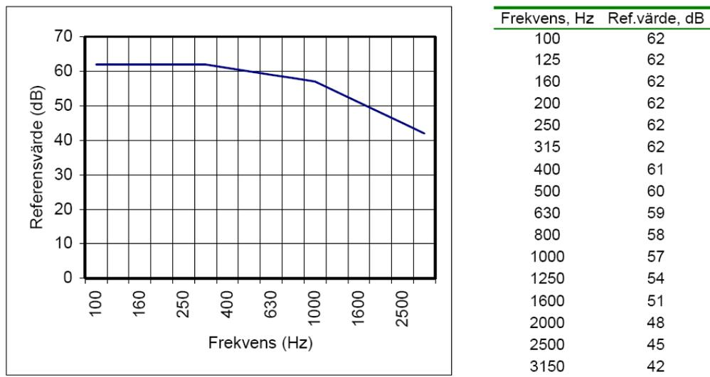
Figure 5 – Reference curve for step sound insulation (ISO 717-2)
