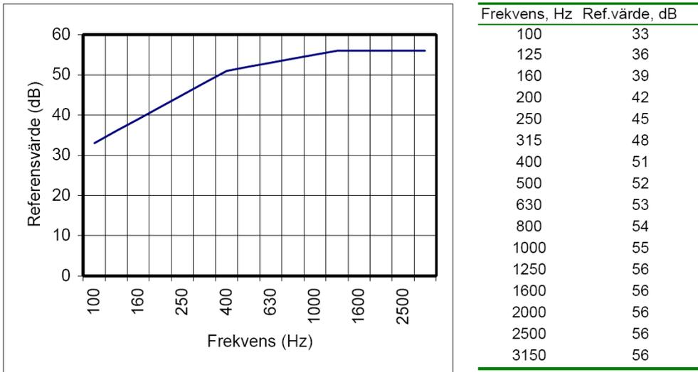
Figure 4 – Reference curve for air borne sound insulation (ISO 717-1)
